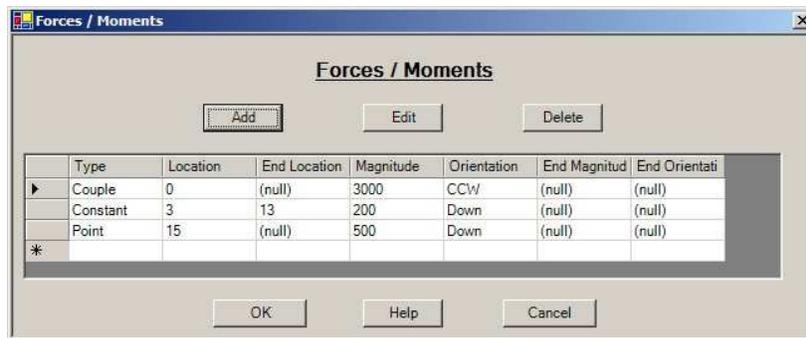
Figure-13: Couple, distributed load, and point load added.
