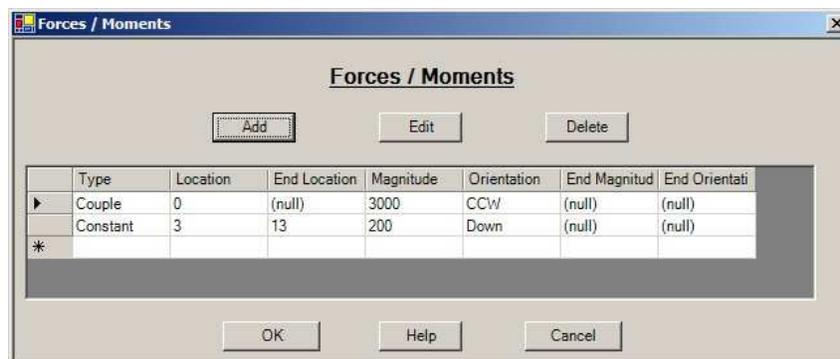
Figure-11: Couple and distributed load added.
